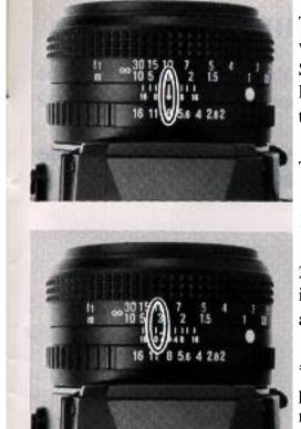
The infrared index mark is an index to correct the focusing point when you use (Black & White film) infrared film and red filters. Since infrared light rays have a longer wave-length than visible light rays, after focusing normally on the subject, you have to set that distance against the infrared index mark.
